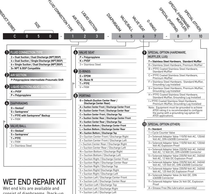
Wet end kits are available and consist of diaphragms, (back-up diaphragms if required), balls, seats and seat O-Rings.
