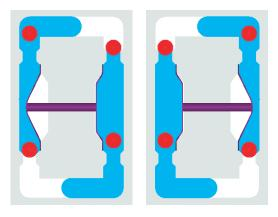
repeated in the opposite direction. In the second figure, liquid is drawn in by the left-hand diaphragm and displaced by the right-hand diaphragm. The liquid is displaced – and thus conveyed – by the compressed air. The diaphragms merely serve as barriers and are not pressurized, this is of critical importance for the service life of the diaphragms.
