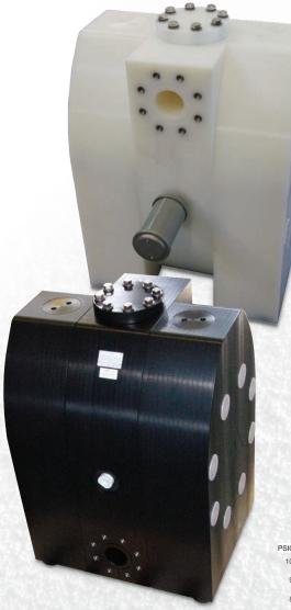
The pump size E 80 extends the E-Series range to seven sizes. With a maximum capacity of 48 m<sup>3</sup>/h the E 80 is proper for an efficient circulation of great quantities. Housing material is PE or PE conductive. The housing bolts are not tighten against a ring. The using of spring washers allows a high security and less leakage liability.
