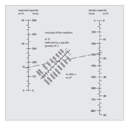
The capacity specified in the pump performance charts generally refers to water (1 mPa·s). The value must be reduced correspondingly when pumping media with higher viscosity. The design capacity can be read off directly from the graph and the corresponding pump size selected.
