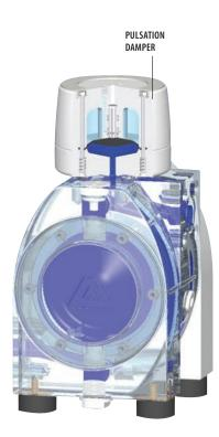
Due to their design, pumps with oscillating action produce a pulsating flow. Although the double-acting design of the E-Series and the direct pneumatic drive have already greatly reduced the pulsation, a pulsation damper must still be installed on the delivery side in order to obtain a virtually uniform flow.
