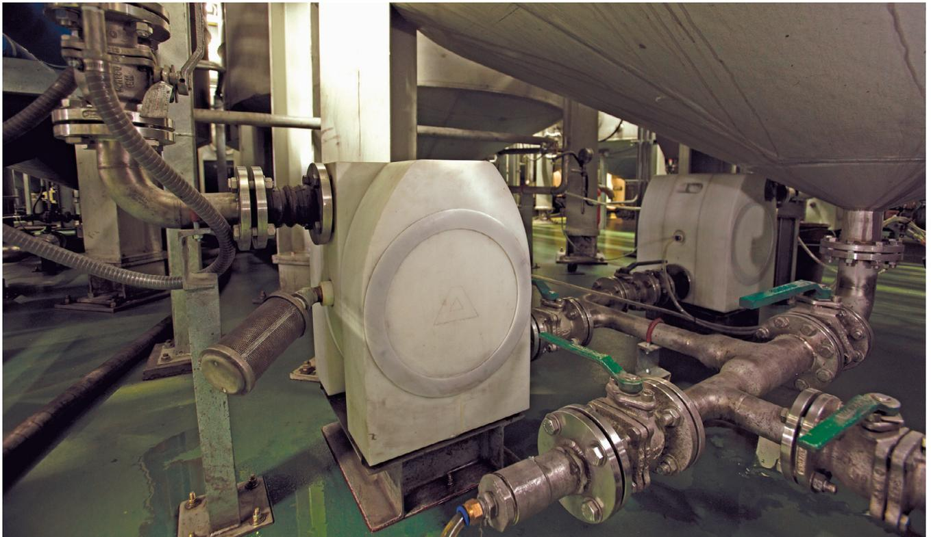
AODD pumps used for transferring abrasive slurry in the solar manufacturing process application.
