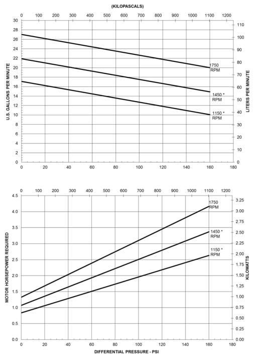
\*1150 and 1450 RPM curves are estimations based on 1750 RPM testing.
