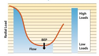
Many processes demand operation off the BEP where higher loads can create damaging vibration.
