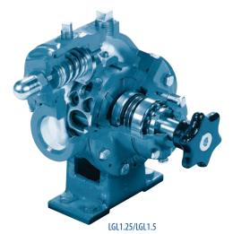
These durable motor speed pumps offer capacities from 9 to 35 U.S. gpm (34-132 L/min), and are ideal for motor fueling, multiple-station cylinder filling and a variety of small transfer jobs. The LGL models are designed for foot mounting to a common base-plate. The LGLF models are fitted with an integral bracket and coupling for direct flange mounting to a NEMA C-face motor. This bracket also allows the pump body to be rotated to simplify hookup to piping systems.
