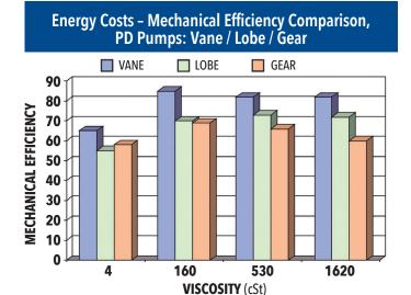
189 - 379 L/min (50-100 GPM); 3.45 - 6.90 Bar (50-100 PSI); 4-1,620 cSt viscosity; same model on all viscosities
