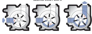
applications, where multi-phase vapor/liquid mixtures are expected. Imagine using the same pump for condensate and crude oil; sliding vane pumps are well suited for both ultra-low viscosity and non-lubricating applications, as well as thick crude applications with suspended solids.
