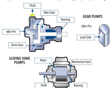
The strain of shaft deflection will cause gear pumps to lose efficiency while sliding vane pumps feature a between-the-bearing design that prevents shaft deflection from occurring.
