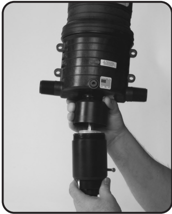
Step 1. Unscrew LOWER END ASSEMBLY from body.
