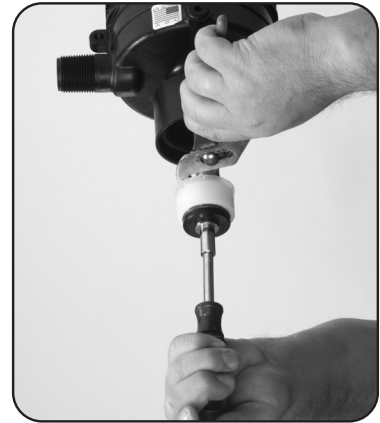
Step 3. Remove #93 CAPSCREW from the end of the shaft using a wrench and nut driver.
