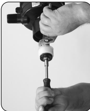
Step 7. Re-install the new #44 DOSAGE PISTON and #73 DOSAGE PISTON GUIDE. Tighten snug using a nut driver.
