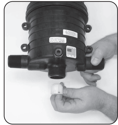
Step 3. Pry the #15 SEAL RETAINER from the injector. Pry #17 O-RING from the unit. NOTE: O-ring may still be seated at the base of the unit.
