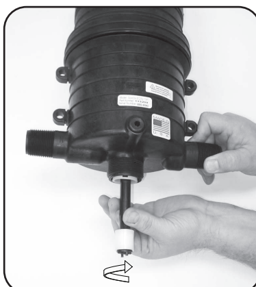
Step 6. Reinsert #51 SHAFT ASSEMBLY into body and rotate 90° to lock. Confirm the shaft is locked in by gently tugging on the shaft. Shaft should remain inserted.
