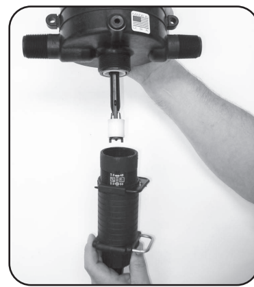
Step 7. Screw LOWER END CYLINDER ASSEMBLY onto body. Ensure #16 gasket is seated on the top of cylinder assembly.
