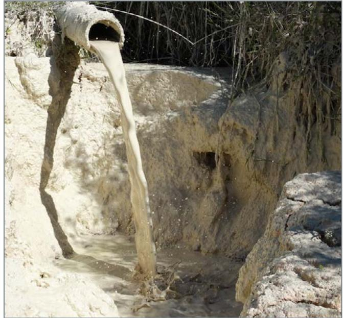
After traveling 800 meters, or half-a-mile, the muddy wastewater is discharged into a retention pond. After the mud settles, the clean water at the top of the pond is reclaimed and reused in the mining process, which helps satisfy the mine’s goal to operate in an environmentally safe and sensitive manner.
