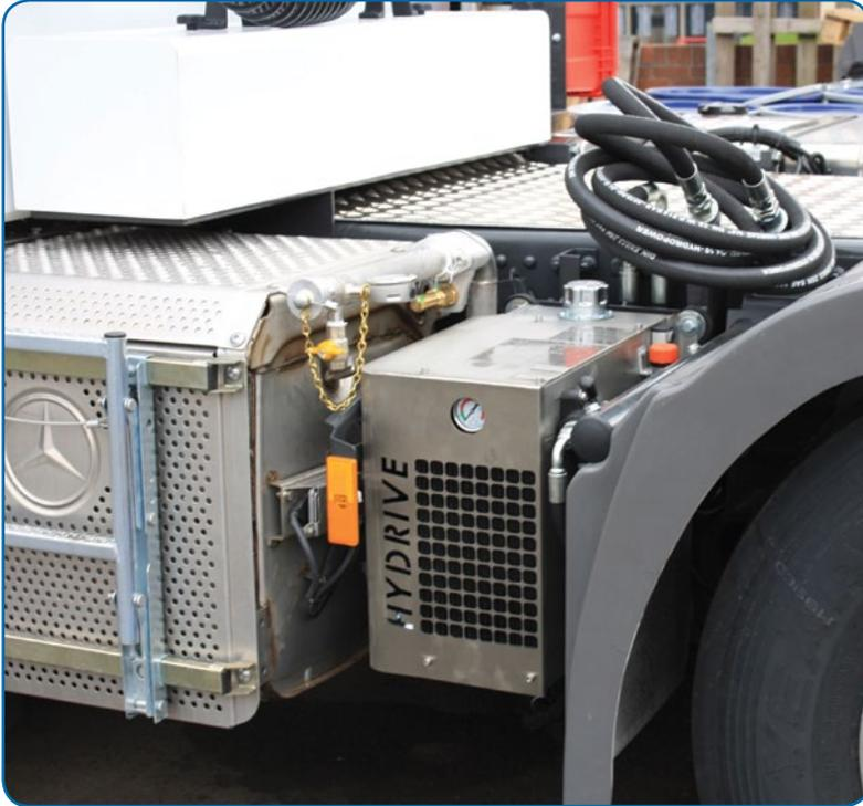
The B200 can be installed as a direct mount, with a PTO, or with a hydraulic drive.
