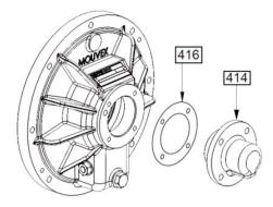
Mounting of front cover bushing in the new bearing.
