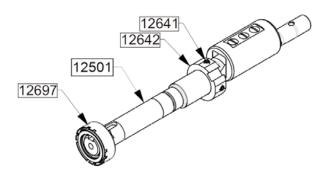
Check shaft 12501 surface condition. Rub it down with thin sand paper if there are scratches on seal rotating part O-ring place. In particular, it must be check that there are no scratches parallel to shaft axis.
