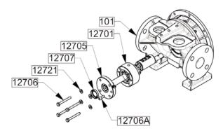
Fit the lip seal 12707, lip orientated outside in the bearing cover 12705.
