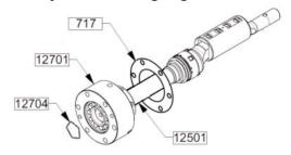
Fit the set bearing cage (12701 - 12703 - 12733 - 12627 and mechanical seal stationary seal face) on the shaft 12501.
