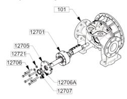
Fit the lip seal 12707, lip orientated outside in the bearing cover 12705.
