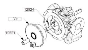
Lubricate the friction surfaces of the piston 301 with a product compatible with the pumped liquid.
