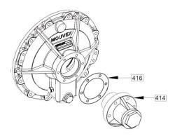
Mounting of front cover bushing in the new bearing.
