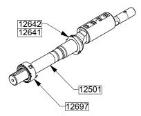
Check shaft 12501 surface condition. Rub it down with thin sand paper if there are scratches on seal rotating part O-ring place. In particular, it must be check that there are no scratches parallel to shaft axis.
