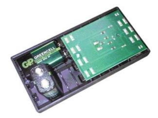
Put back batteries by the opposed side to connections and press them down.
