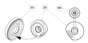
Place thread locking adhesive (Loctite<sup>®</sup> 243\* or equivalent) on the thread of the transmission hub 596.
