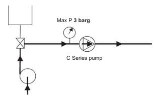
It is preferable not to run the C Series pump during CIP although low speed (< 100 rpm) is acceptable by alternating start/stop operation.
