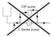
Indeed, in this case, the pressure at the inlet of the C Series pump is lower than the pressure at the discharge and the piston remains forced against the cylinder. Therefore, there the C Series pump no longer provides a passage. Its efficient cleaning can no longer be ensured and the cylinder/piston pair will become prematurely worn.
