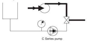
The C Series pump is stopped when cleaning the installation.
