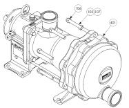
• Remove the front cover **401** with the 2 screwdrivers. If the discharge piping is mounted in a rigid manner, pivot the bottom **401** so as to free the connection.
