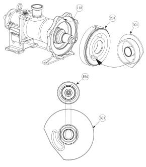
• Place thread locking adhesive (Loctite<sup>®</sup> 243\* or equivalent) on the thread of the transmission hub **596**.
