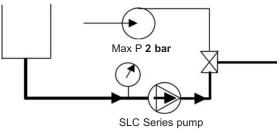
We recommend limiting the rotation speed of the SLC Series pump.
