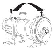
• Screw the lifting hook in the tapped hole of the cylinder, provided for this purpose and tighten the screw in the location of the lifting ring.
