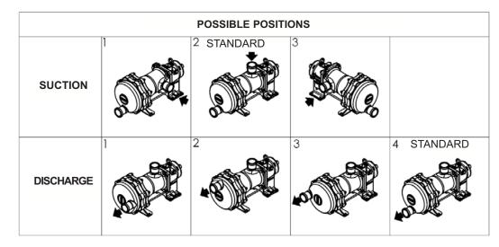
The SLC Series pump is a selfpriming volumetric PD pump.
