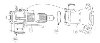
Assembly is undertaken in the reverse order of dismantling, taking care to correctly position the seal 113 and the indexing pin 513. The nuts 115 must be re-mounted with thread locking adhesive (Loctite<sup>®</sup> 243\* or equivalent) : 4 x M16 : Assembly torque 75 Nm. Under preventive maintenance (every 135 millions of cycles duty) or in case of damage of the bellows, we suggest transmission exchange program.
