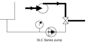
The SLC Series pump is stopped when cleaning the installation.
