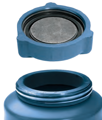
NEPTUNE HIGH-PRESSURE CAP Coarse thread, 2-1/2 turn design rated to 300 psi.
