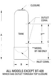
\*4" (102 mm) : Closure with 1" NPT connection for piping.
