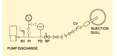
the maximum operating pressure. The relief valve return is piped back into the tank. Transparent return tubing allows fluid to be observed in the line if the relief valve opens. When portable, replaceable containers are used as the chemical source, it is convenient to pipe the relief valve back into the suction line. When piping the relief valve return to the suction, be certain the return is upstream of the pump suction isolation valve so that the flow path back to the tank cannot be blocked.
