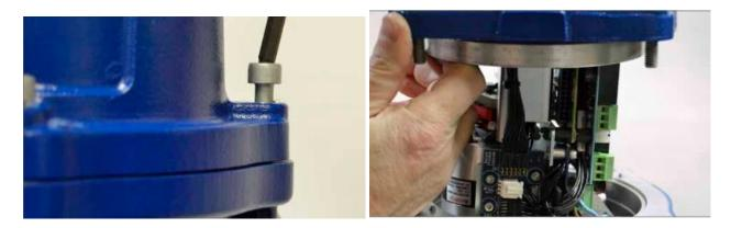
Using a 6 mm Allen key loosen the captive fixings securing the terminal compartment cover. Do not attempt to lever off the cover with a screwdriver as this will damage the o-ring seal and may damage the flamepath on a certified unit.
