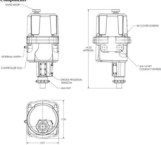
**Handwheel Operation** The handwheel is located on the top cover. Push and hold the handwheel down and rotate to extend/retract or rotate the actuator output drive. Verify direction of output shaft rotation for clockwise operation of the handwheel. Stroke position can be found at the local display window
