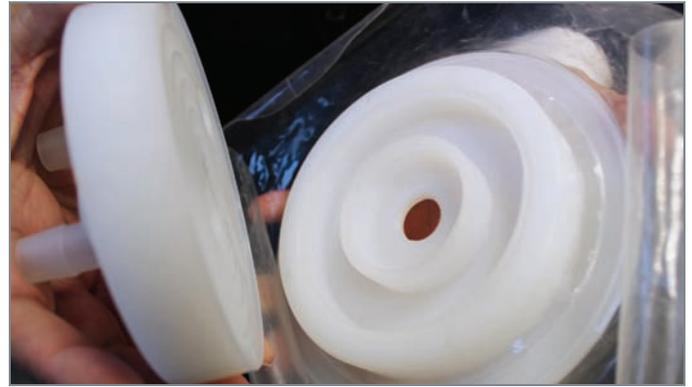
The QuattroMix™ system has a very basic, easy-to-understand operating principle and includes a single-use mixing bag, a Quattroflow™ pump and a 16-hole mixing plate that is built into the bag.
