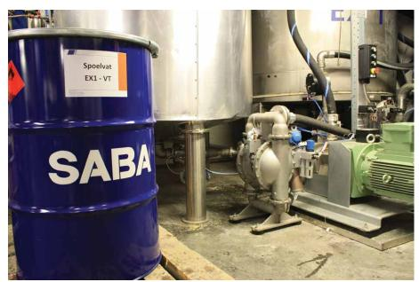
SABA Dinxperlo B.V. has grown into one of the world's largest independent producers of adhesives and sealants by identifying the challenges in product manufacture and handling, and choosing the technology that makes the process as safe as possible. Wilden® AODD pumps help optimize the process, from raw-material transfer to the packaging of finished end-products.
