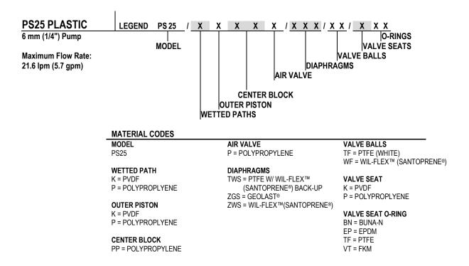
! NOTE: Most elastomeric materials use colored dots for identification
