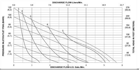
Flow rates indicated on chart were determined by pumping water. For optimum life and performance, pumps should be specified so that daily operation parameters will fall in the center of the pump's performance curve.
