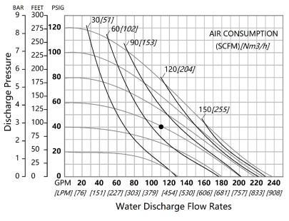
**Example:** A PR1560 metal rubber-fitted pump achieved a flow rate of 416lpm (110 gpm) using 127.5Nm<sup>3</sup>/h (75 scfm) of air when run at 4.1bar (60 psi) air inlet pressure and 2.7 bar (40 psi) discharge pressure. Flow rates indicated on chart were determined by pumping water. For optimum life and performance, pumps should be specified so that daily operation parameters will fall in the center of the pump's performance curve.
