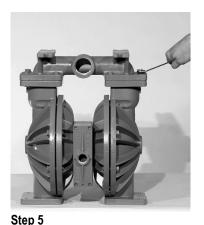
Remove the hardware attached to inlet manifold and liquid chambers.
