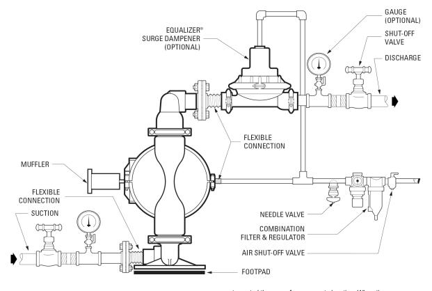
**NOTE:** In the event of a power failure, close the shutoff valve if you do not want the pump to restart when the power returns.
