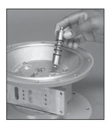
Step 7 Remove pilot spool sleeve from center section.
