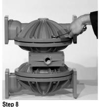
Remove the hardware attached to liquid chamber.
