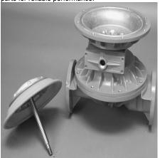
**Step 10** After loosening and removing the outer piston the diaphragm assembly can be disassembled.
