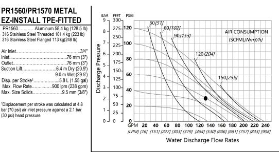
Example: A PR1560 metal EZ-Install Wil-Flex-fitted pump achieved a flow rate of 492 lpm (130 gpm) using 127.5Nm3/h (75 scfm) of air when run at 4.1 bar (60 psi) air inlet pressure and 2.1 bar (30 psi) discharge pressure.
