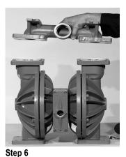
Remove the inlet manifold and Inspect ball cage area of manifold for excessive wear or damage.
