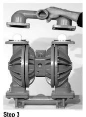
Lift the discharge manifold and Inspect ball cage area of manifold for excessive wear or damage.
