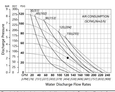
Flow rates indicated on chart were determined by pumping water. For optimum life and performance, pumps should be specified so that daily operation parameters will fall in the center of the pump's performance curve.
