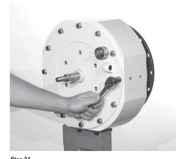
Using a socket wrench, unbolt the power cylinder cover from the center section.
