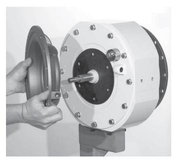
**Step 23**Remove the air chamber fasteners and gasket.
