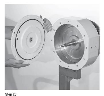
This will force the power cylinder cover away from the power cylinder body. Inspect shaft bushing seals and O-ring on power cylinder cover for damage.
