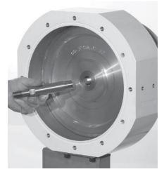
**Step 28**Remove the outer piston, diaphragm and shaft assembly from the air chamber.
