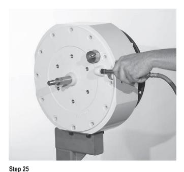
Using an air nozzle with a rubber tip, apply air to the air manifold tube port.
