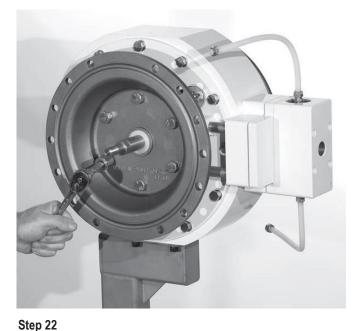
Using the appropriate-sized wrench, remove the air chamber fasteners.
