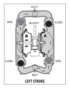
**FIGURE 3** At completion of the stroke, the air valve again redirects air to the back side of diaphragm A, which starts diaphragm B on its exhaust stroke. As the pump reaches its original starting point, each diaphragm has gone through one exhaust and one discharge stroke. This constitutes one complete pumping cycle. The pump may take several cycles to completely prime depending on the conditions of the application.
