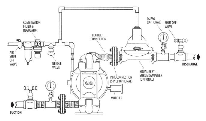
Air Operated Pumps: To stop the pump from operating in an emergency situation, simply close the "shut off" valve (user supplied) installed in the air supply line. A properly functioning valve will stop the air supply to the pump, therefore stopping output. This shut off valve should be located far enough away from the pumping equipment such that it can be reached safely in an emergency situation.
